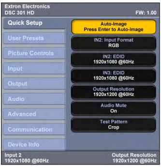
Figure 3. OSD Menu – Quick Setup Submenu
